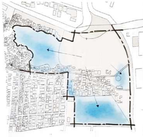
MAXIMUM RAIN WATER IS COLLECTED ON LAND WITH MAXIMUM VEGETATION DUE TO LOWEST LYING CONTOURS
