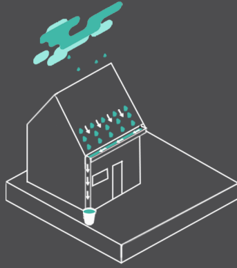
Rainwater harvesting [16] 50,000 m 2 of roof - ≈ 138.888 L/year
