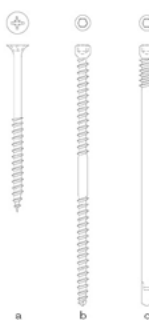
Self-tapping connectors: a Spax self-tapping screw b Double-thread screw c Self-drilling dowel
